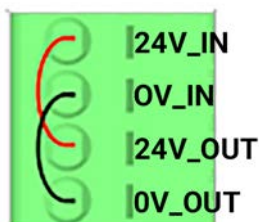
Figure 30: Internal power supply terminal connections
