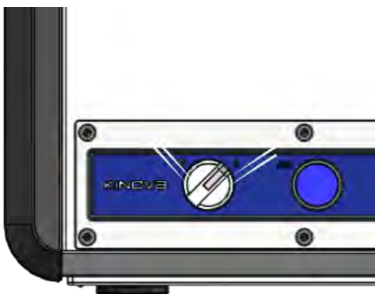
Figure 43: Visual cues for controller initialization
