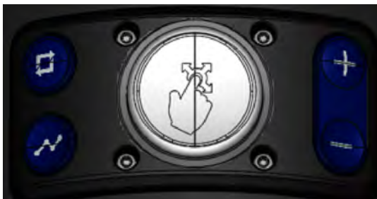
Figure 54: Center button on the wrist is the Wrist enabling device button
