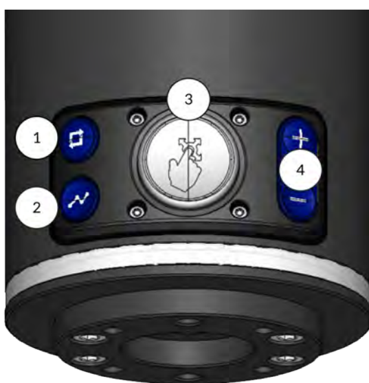
Figure 12: Buttons on the wrist
