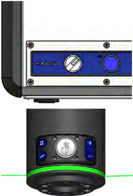
Figure 47: Visual cues of robot in Monitored stop
