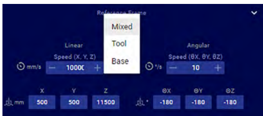
Figure 149: Available frames of reference in the Jog Cartesian panel
