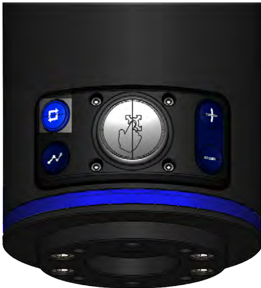
Figure 56: Location of Teach mode toggle on the wrist
