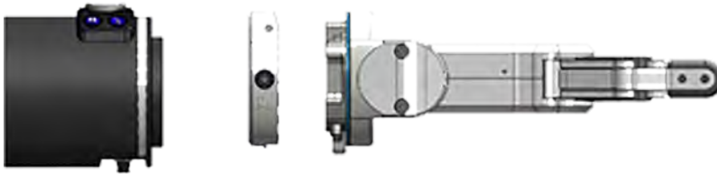
Figure 190: Wrist, flange, OnRobot ISO adapter, and OnRobot RG2 Gripper
