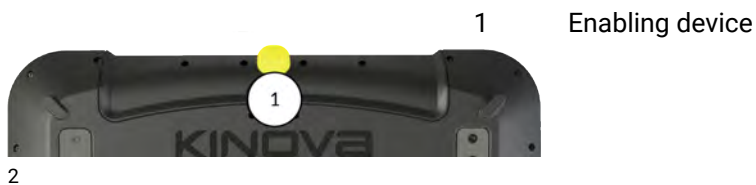
Figure 52: Location of enabling device on the teach pendant
